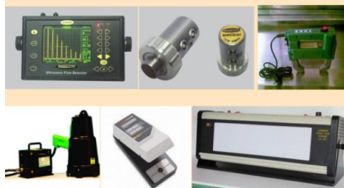
Digital Ultrasonic Flaw Detector, Magnetic Particle Testing Equipment, calibration blocks and flawed specimens, Dye penetrant Testing kit & flawed specimens, Radiography accessories funded by Sathyabama
