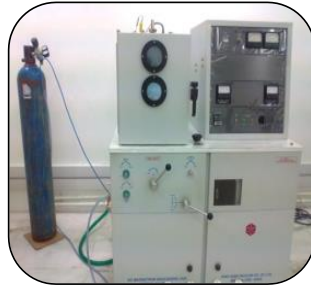
DC Magnetron Sputtering System Model 12" MSPT Box type
