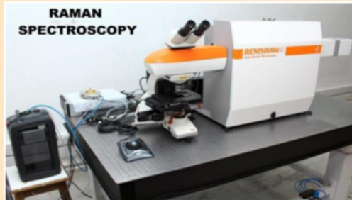
RENISHAWinVia Confocal Raman microscope (United Kingdom) funded by Sathyabama Institute of Science and Technology
