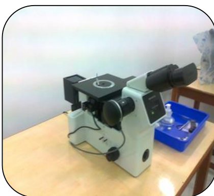
Inverted Metallurgical Microscope, Model GX71, Olympus, Japan
