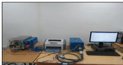
Potentiostat/ Galvanostat with Impedance Analyzer- Bio-Logics, France
