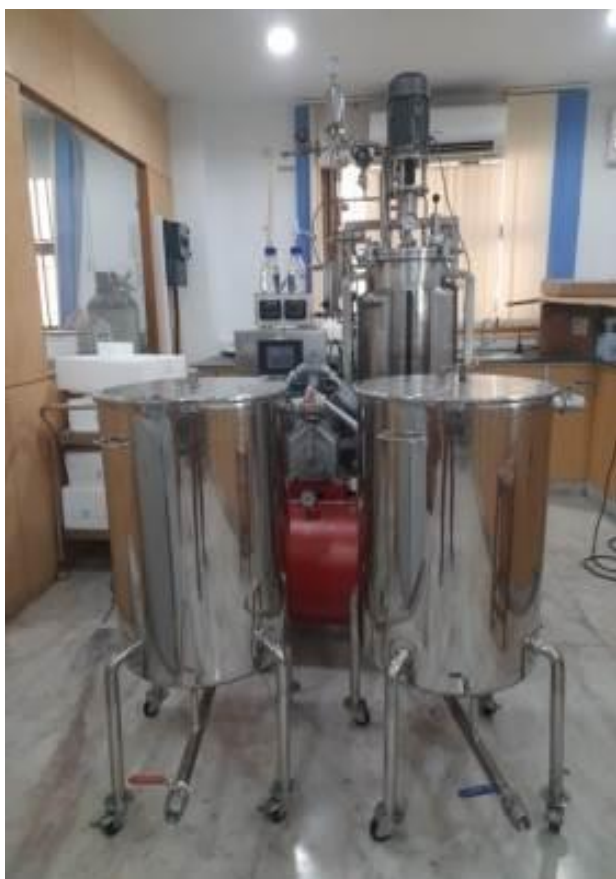
SS Extraction unit
