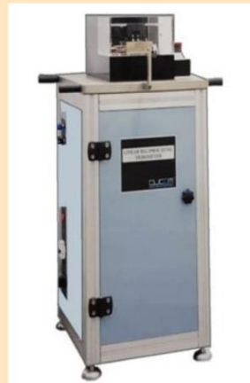
Linear Reciprocating Tribometer (LRT) funded by DST-SERB
